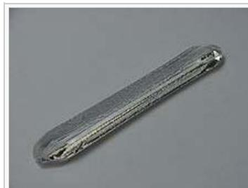
A synthetic quartz crystal grown by the [hydrothermal method](#), about 19 cm long and weighing about 127 grams
