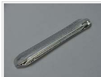
A synthetic quartz crystal grown by the hydrothermal method , about 19 cm long and weighing about 127 grams
